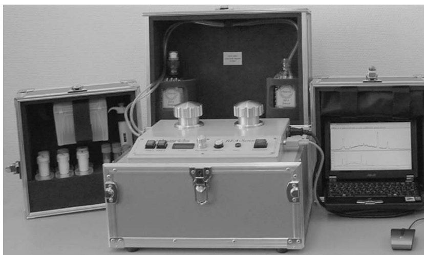
Fig. 1. X-ray fluorescence analyzer with a sorption accumulation microsystem.
