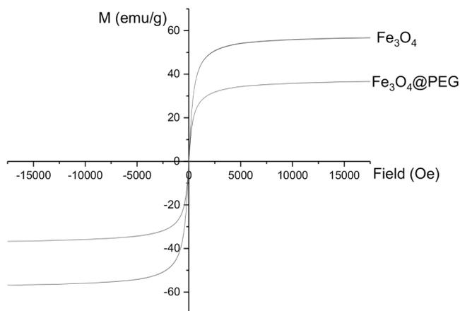
Fig. 2. Magnetization curves for  $\text{Fe}_3\text{O}_4$  and  $\text{Fe}_3\text{O}_4@PEG$  samples.
