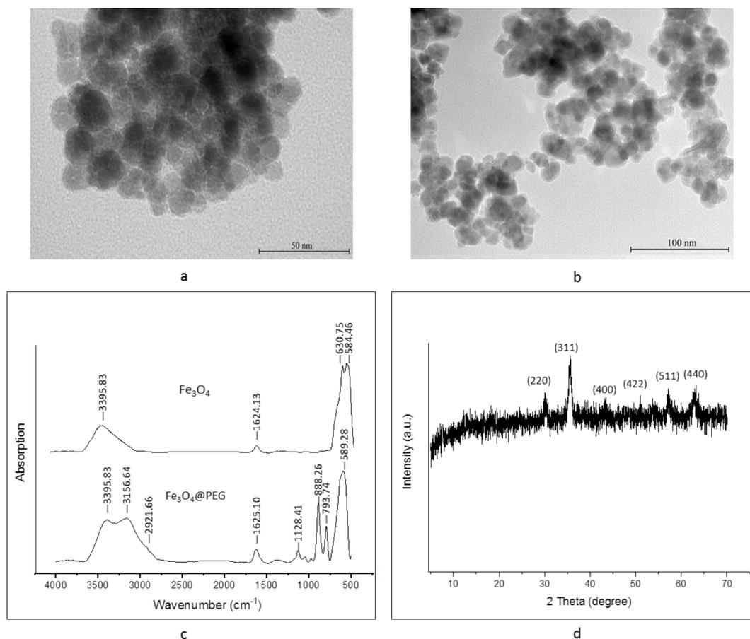
Fig. 1. TEM images for Fe<sub>3</sub>O<sub>4</sub> (a) and Fe<sub>3</sub>O<sub>4</sub>@PEG (b), FT-IR spectra for Fe<sub>3</sub>O<sub>4</sub> and Fe<sub>3</sub>O<sub>4</sub>@PEG (c) and XRD pattern for Fe<sub>3</sub>O<sub>4</sub>@PEG (d).
