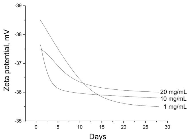
Fig. 3. Change of zeta-potential for  $\text{Fe}_3\text{O}_4@PEG$  MNPs over time.
