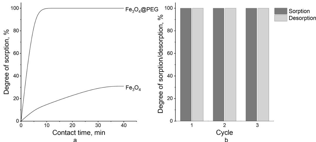
Fig. 4. Degree (%) of LO sorption by  $\text{Fe}_3\text{O}_4$  and  $\text{Fe}_3\text{O}_4@PEG$  MNPs (a); degree (%) of LO sorption/desorption by  $\text{Fe}_3\text{O}_4@PEG$  MNPs during 3 cycles (b).
