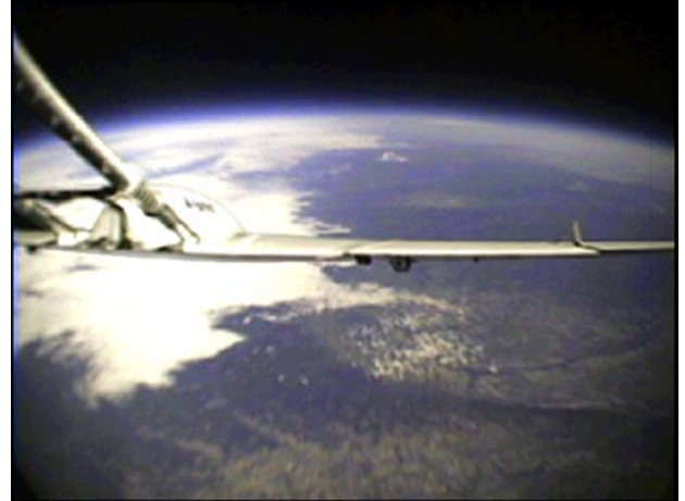
Figure 3. Video still from the successful deployment of a half-scale model of ARES at Mars-relevant atmospheric pressure above Oregon, USA.
